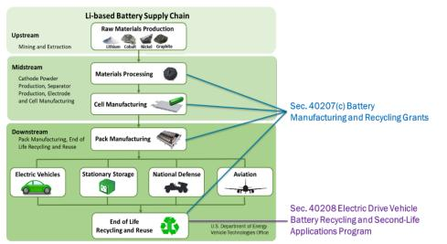
The high-capacity battery supply chain consists of five main steps: (1) raw material production, (2) materials processing including material refinement and
