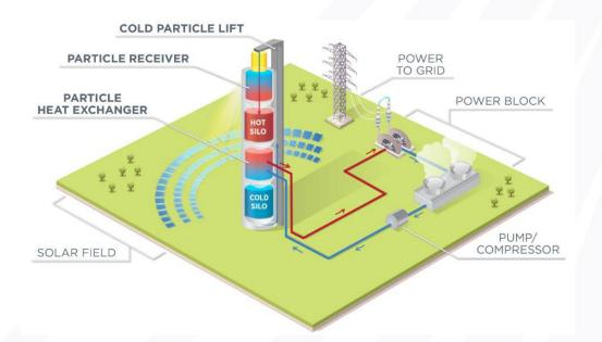
Figure above shows the general design of a particle based CSP system; several forms of particle receiver shape, design and layout of silos, heat exchanger and intermediate lift are feasible; power block is a representation
