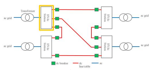
**Figure 1:** A high-level representation of a generic multi-terminal HVDC VSC system. Multi-terminal systems provide increased reliability and redundancy of the system, as well as provide multiple avenues for the electricity to flow based on grid need.
