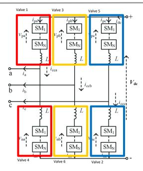
**Figure 2:** A MMC VSC is composed of 6 valves as indicated by the red, yellow, and blue boxes. Each valve has many submodules dependent on the power rating of the converter. Valves 1, 3, & 5 process the positive phases of AC current and valves 2, 4, & 6 process the negative phases.
