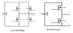
**Figure 3:** The full-bridge and half-bridge configurations are depicted as a and b, respectively. Half-bridge submodules contain half the number of IGBTs as the full bridge, making half-bridge submodules the less expensive configuration by nearly half.
