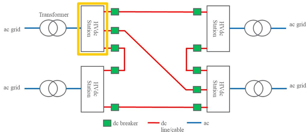
**Figure 1:** A high-level representation of a generic multi-terminal HVDC VSC system. Multi-terminal systems provide increased reliability and redundancy of the system, as well as provide multiple avenues for the electricity to flow based on grid need.
