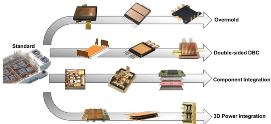
Figure 21. Advanced power module designs for SiC [16]
