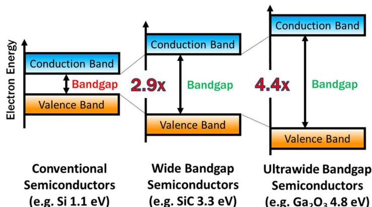
Figure 3. Energy bandgap comparison of conventional semiconductors (e.g., Si), WBG (e.g., SiC), and UWBG (e.g., gallium oxide)
