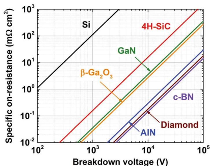
Figure 4. Contours of constant Baliga figure-of-merit (BFOM) showing relationship between on-resistance and breakdown voltage for various conventional, WBG, and UWBG semiconductors<sup>11</sup>
