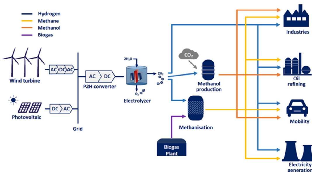
Figure 11. Architecture of power-to-hydrogen (P2H) with renewable energy input for industrial utilization<sup>47</sup>
