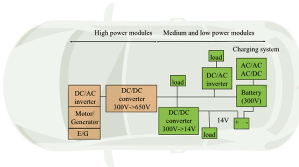
Figure 8. PE components in a BEV<sup>39</sup>
