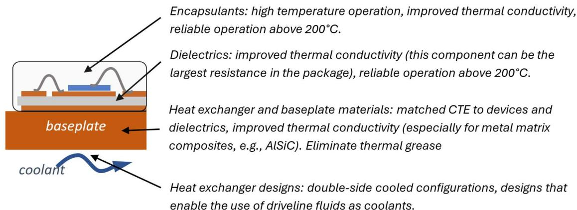
Figure 19. Power device package with associated requirements
