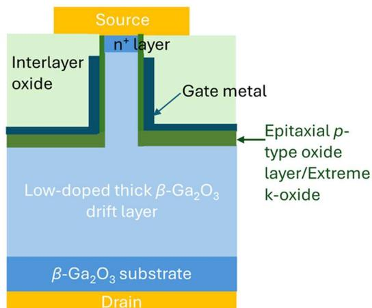
Figure 16. Schematic of vertical  $\beta\text{-Ga}_2\text{O}_3$  based transistor<sup>184</sup> employing an integrated epitaxial p-type layer (JFET) or an extreme k-dielectric oxide (MOSFET) towards  $> 5\text{kV}$  breakdown voltages
