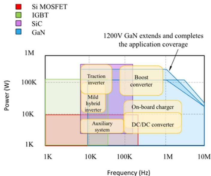
Figure 9. Power vs frequency comparison of different semiconductor technologies for EV power converters<sup>40</sup>
