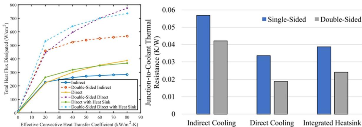
Figure 20. Comparison of heat flux capacity and thermal resistance of different cooling designs<sup>245</sup>
