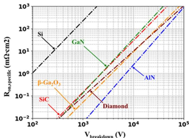
Figure 15. Calculated unipolar figure of merit lines for Si and several WBG and UWBG semiconductors<sup>146</sup>
