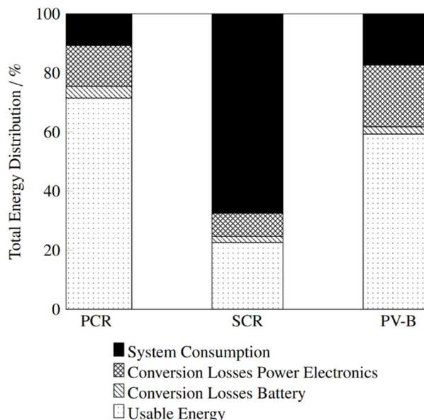
Figure 6. Losses in Battery Energy Storage Systems (BESSs)<sup>22</sup>
