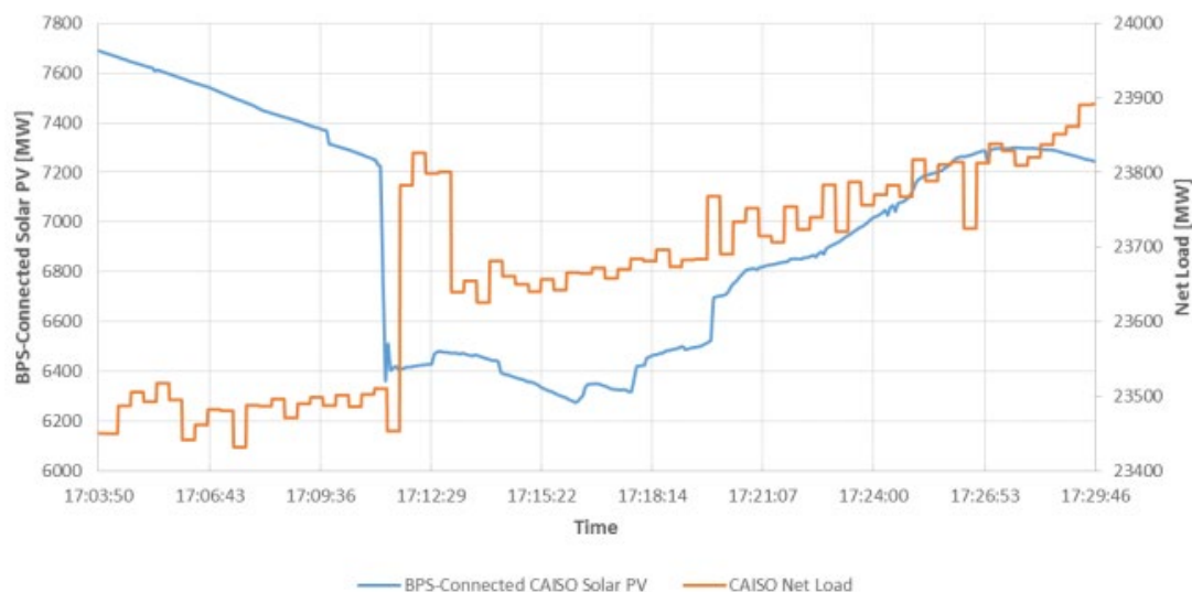
Figure 7. Fault scenario in which large, metered solar generating plants cease production during a disturbance, and distributed PV generation simultaneously stops producing, which contributes to a sudden increase in net load. 57
