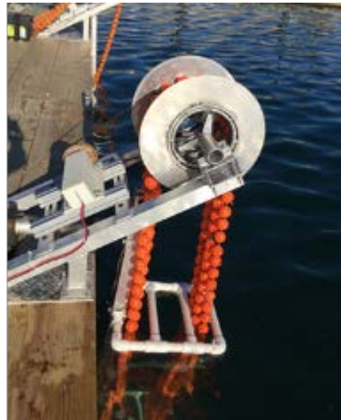
Figure 36. Adsorbent material encapsulating in a protective sphere (left), and symbiotic machine for ocean uranium extraction (right). Source: Haji et al. 2017a
