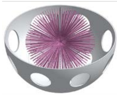
Figure 36. Adsorbent material encapsulating in a protective sphere (left), and symbiotic machine for ocean uranium extraction (right). Source: Haji et al. 2017a
